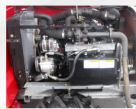
54 horsepower diesel engine
